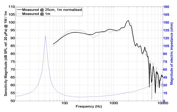
HD curve measured on CEI standard baffle :
